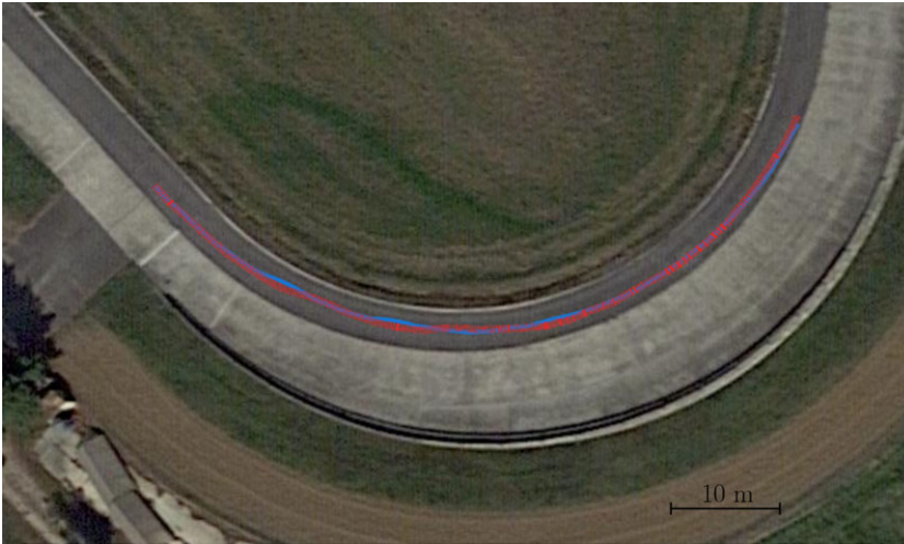
Figure 13. Comparison between measured (dashed red line) and simulated path (solid blue line) followed by the robot during the validation test on a curved path. GPS coordinates of the test site (DMS format): 44° 57' 24.5988" N, 7° 33' 25.956" E).
