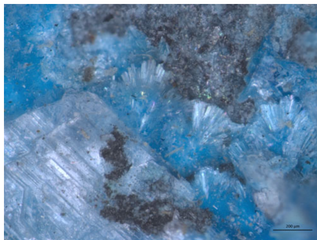
Fig. 1. Close-up of acicular bridgesite-(Ce) crystals on cotype sample BM 2007,82. The scale bar is 200 µm and the associated colourless crystal to the bottom left is gypsum.
