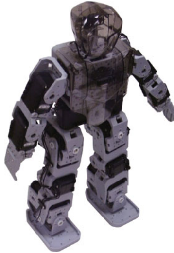
Fig. 3. The 18-DOF humanoid robot whose model is used for simulations.
