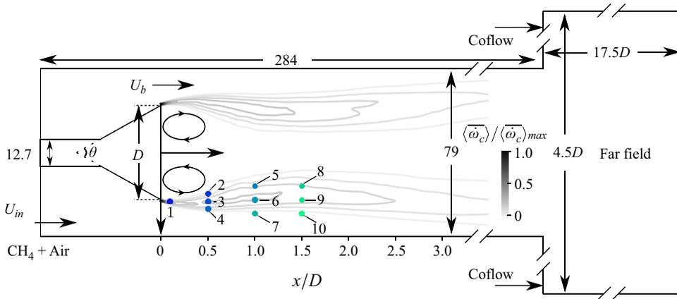
Figure 2. Schematic of the bluff-body burner (Pan *et al.* 1990; Nandula 2003). Time series data for all quantities are extracted from the ten probe locations indicated. The contour lines denote the time-averaged reaction rate of progress variable  $\bar{\omega}_c$  normalised by its maximum value. All dimensions are in mm.
