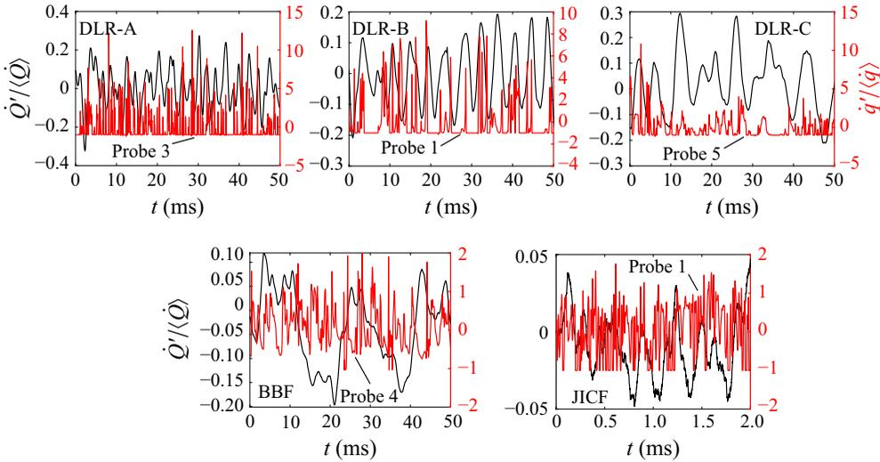
Figure 5. Time series  $\dot{Q}'$  and  $\dot{q}'$  normalised by their respective time averages for cases DLR-A, DLR-B, DLR-C, BBF and JICF. The typical local HRR data are shown for arbitrary probe locations indicated.
