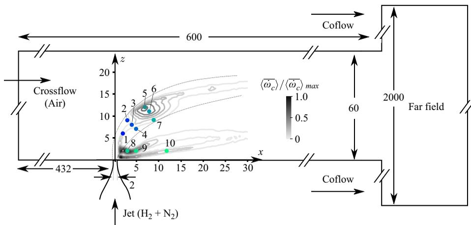
Figure 3. Schematic of the JICF burner (Steinberg *et al.* 2013). Time series data for all quantities are extracted from the ten probe locations indicated. The contour lines denote the time-averaged reaction rate of progress variable  $\bar{\omega}_c$  normalised by its maximum value. All dimensions are in mm.
