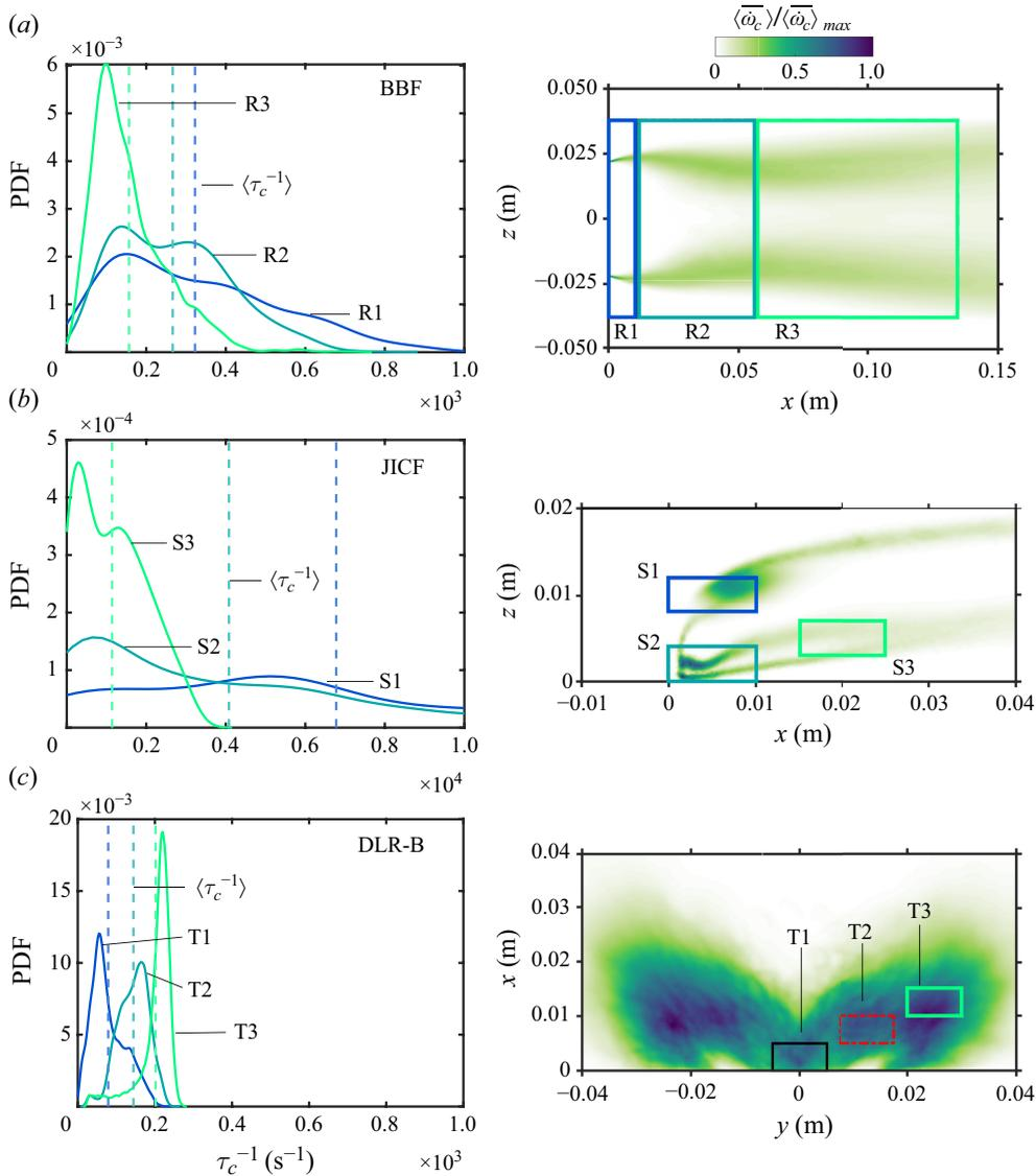
Figure 10. The PDFs of  $\tau_c$  for three spatial zones marked in the right-hand column showing  $\langle \overline{\dot{\omega}_c} \rangle / \langle \overline{\dot{\omega}_c} \rangle_{max}$ . The dashed vertical lines indicate the mean  $\tau_c^{-1}$  in each zone.
