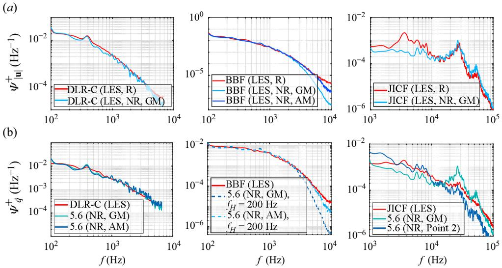
Figure 16. (a) Comparison of mean reacting (R) and non-reacting (NR)  $\psi_{|u|}^+$ , and (b) comparison of LES results and model (5.6), using normalised NR velocity magnitude PSD for DLR-C, BBF and JICF. Here, AM means arithmetic mean, and GM means geometric mean.
