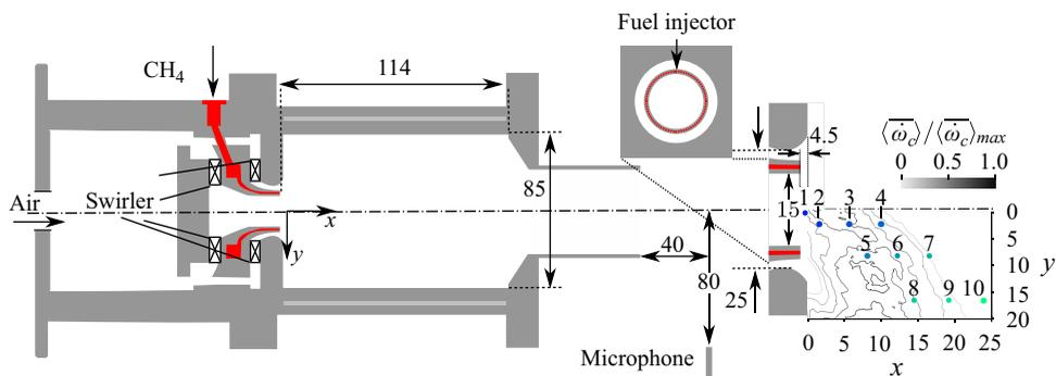
Figure 1. Schematic of the dual-swirl gas turbine model combustor (Meier *et al.* 2006; Weigand *et al.* 2006). Time series data for all quantities are extracted from the ten probe locations shown. The contour lines denote the time-averaged reaction rate of progress variable  $\bar{\omega}_c$  normalised by its maximum value. All dimensions are in mm.
