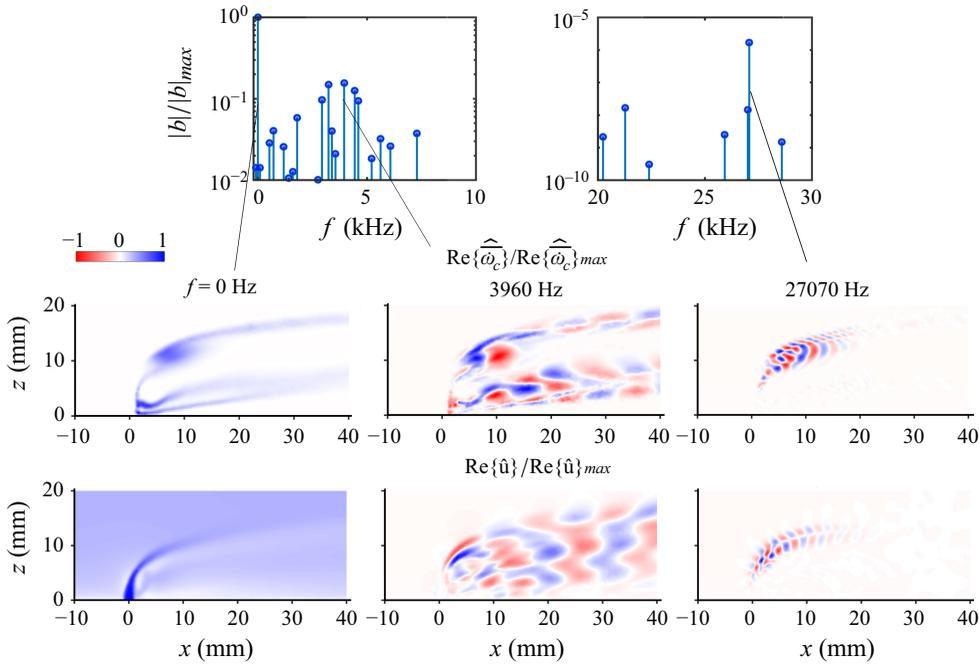
Figure 9. The DMD mode amplitude of  $\widehat{\omega}_c$  and  $|\mathbf{u}|$  for the JICF flame, and the spatial distribution of three modes.
