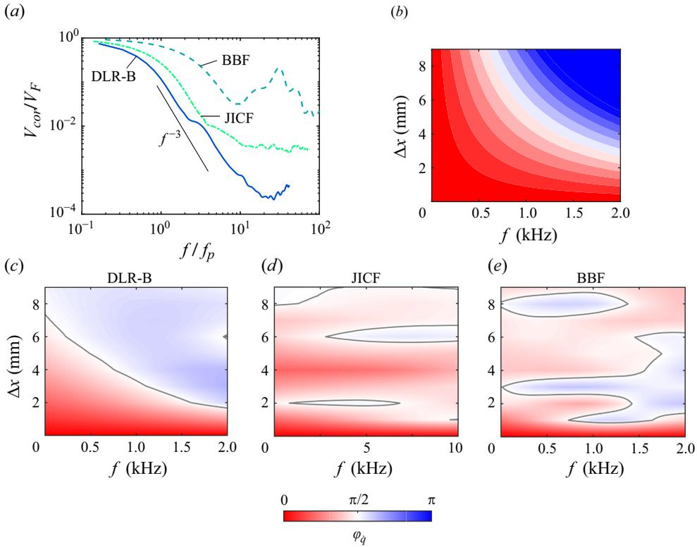
Figure 11. (a) The frequency spectrum of the correlation volume normalised by the flame volume  $V_F$ . (b–e) Contours of cross-spectrum phase  $\varphi_{\dot{q}}$  of transversely integrated HRR along  $(y, z)$  for a synthetic signal and cases DLR-B, JICF and BBF. Grey contour lines denote the mark  $\varphi_{\dot{q}} = \pi/2$ .
