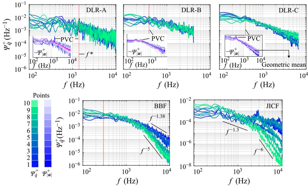
Figure 7. The variation of  $\psi_q^+$  with  $f$  at ten probe locations for the five cases. The insets in the DLR cases show the normalised PSD of velocity magnitude,  $\psi_{|u|}^+$ , for the same probe locations. The magenta line shows the geometric mean of  $\psi_{|u|}^+$  at the ten probe locations. The vertical red dotted line marks the characteristic frequency  $f^*$ .
