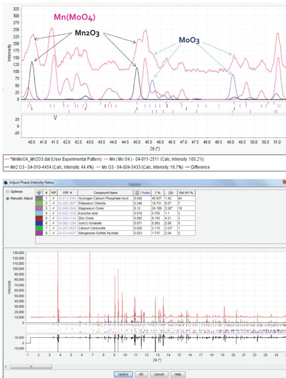
Figure 5. (Color online) Identification of materials from a constant wavelength neutron diffraction experiment (top) and a synchrotron diffraction experiment (bottom). Each module has an ability to import experimental data and match it to reference data that has been modified for instrument type, detector (1D or 2D), wavelength, and radiation type.
