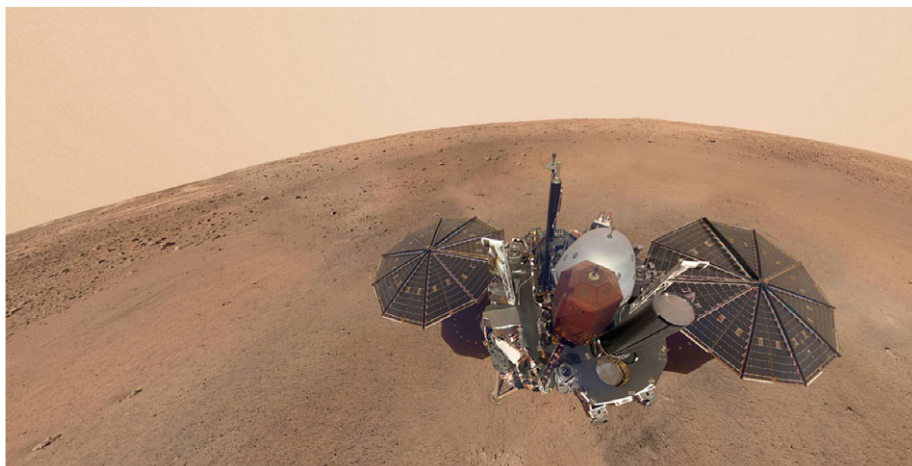
Figure 1. A selfie from Mars, built with composite images from the IDC camera, showing the InSight lander before the deployment of SEIS on the ground. (Source NASA; https://mars.nasa.gov/insight/resources/22211/insights-first-selfie/ ).
