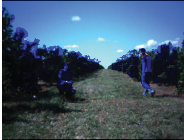
Fig. 10. Comparison between the results of the “full” CPU implementation and a projected one with a frame of the stereo log. Blue pixels represent obstacles detected by both implementations and red pixels are the ones detected only by the “full” CPU implementation.
