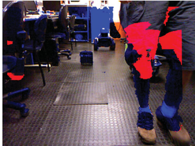
Fig. 11. Comparison between the results of the “full” CPU implementation and GPU Kernel 1 one with a frame of the kinect log. Blue pixels represent obstacles detected by both implementations and red pixels are the ones detected only by the “full” CPU implementation. This is not the case of the proper projected implementations (i.e. single-core, multi-core and Kernel 3 ).
