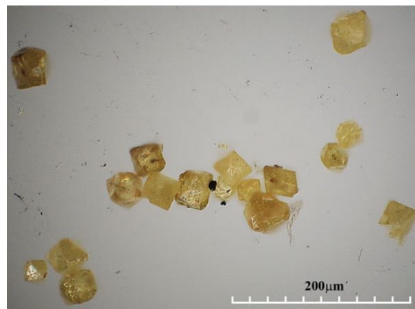
Fig. 2. The crystal forms of hydroxyplumbopyrochlore.
