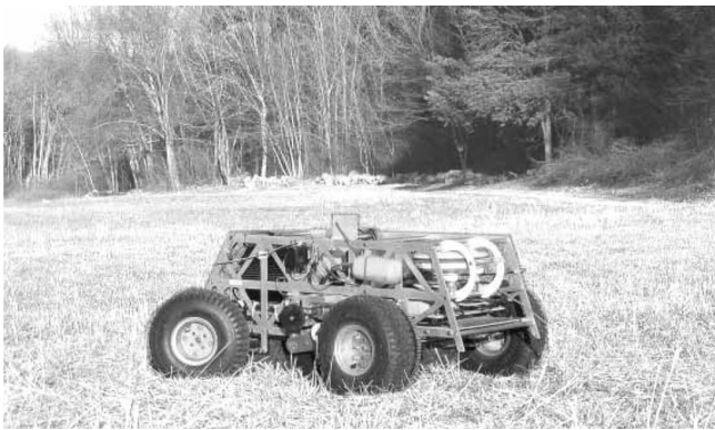
Fig. 31. ARTEMIS experimental UGV on outdoor terrain.
