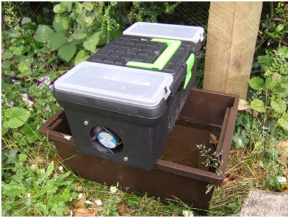
Fig. 1. Gravid box trap based on Reiter gravid box trap design (Reiter, 1987).
