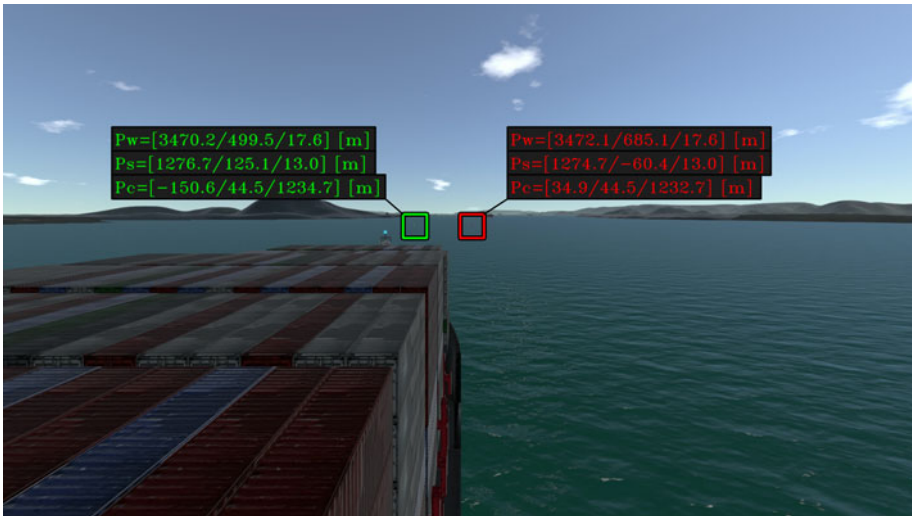
Figure 10. Simple highlighting for each buoy with a summary of coordinates expressed in different frames.
