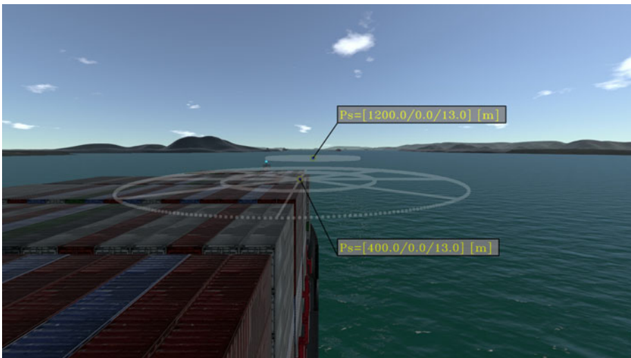
Figure 15. Circular highlight representing waypoints of the expected trajectory for the ship in the simulation.
