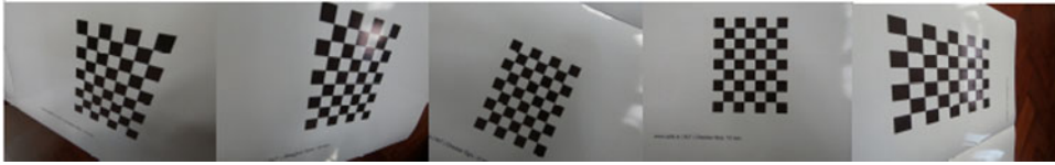
Figure 2. Observation of known planar patterns for calibration.
