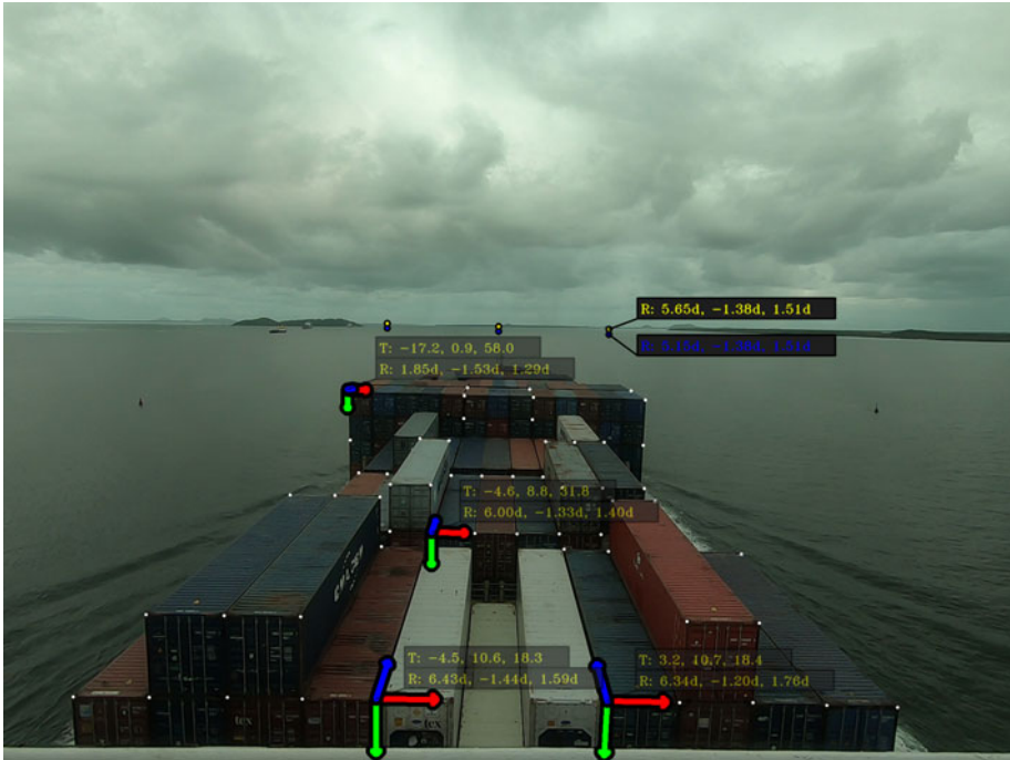
Figure 9. Camera calibration with visible points from onboard containers.
