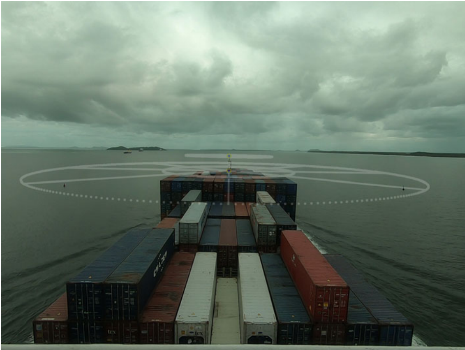
Figure 16. Circular highlight representing waypoints of the expected trajectory for the ship in reality.
