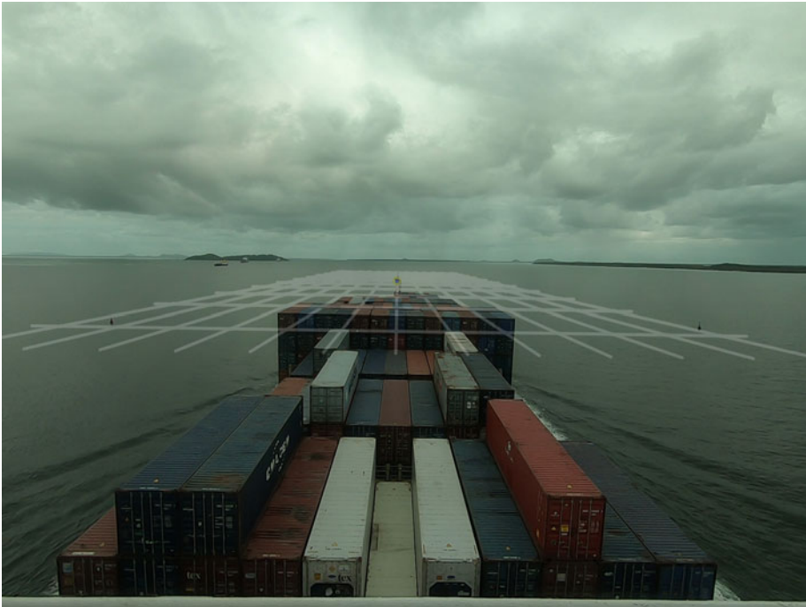
Figure 21. Auxiliary rectangular grid for estimating the relative position of surrounding obstacles in reality. Each rectangle of the grid has dimensions 100\text{ m} \times 25\text{ m} .
