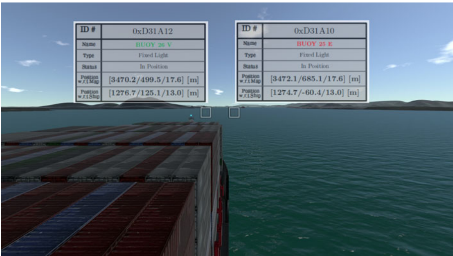
Figure 17. Information highlight for each buoy in the simulation.
