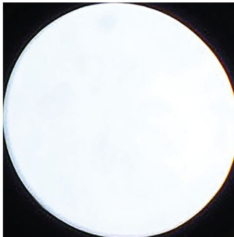
Figure 4. Reflection of the collimated light source as seen by the camera for a perfectly flat interface.
