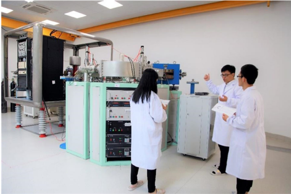
Figure 2 A single-stage 200 kV AMS system at GXNU.
