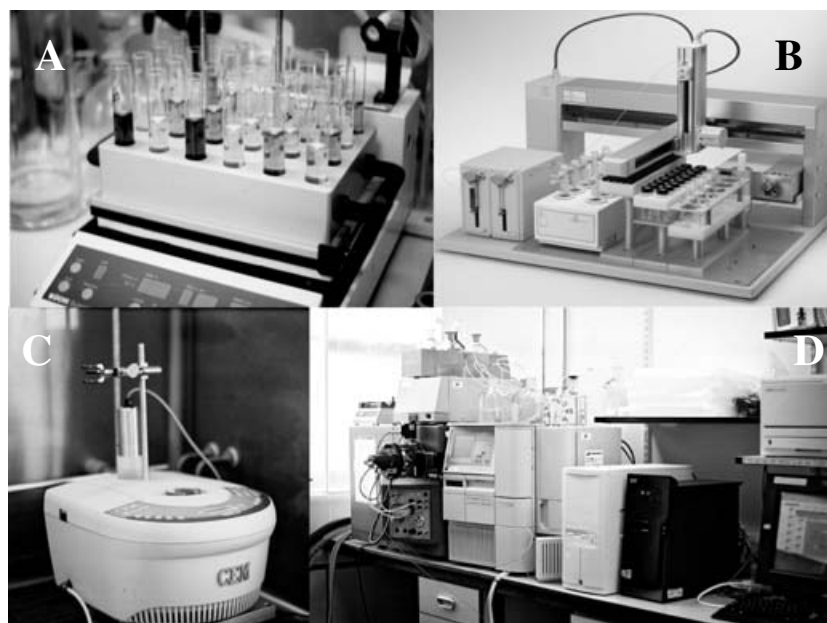
Fig. 3. Chemical technology that aids protein target identification. The main goal of this technology is to increase the rate of analogue synthesis enabling the rapid acquisition of structure activity relationship (SAR) data (Hird, 1999). Images A–D show examples of the technology used in our research group. A and B: semi- and fully-automated reaction blocks often supplied with filtration and separation devices, enabling both solid and solution phase chemistry. Maximum use of these systems requires automated purification systems (up to 10 compounds can be purified in parallel, equipment not shown); C: focused microwave apparatus. This technology enables reactions that have been traditionally carried out on the time scale of hours to be carried out in minutes. For a recent application from our laboratory see Patterson et al. (2004); D: automated analytical systems. The liquid chromatography-mass spectrometry system shown here enables the assessment of compound purity and structure 24 hours a day. Additional analytical techniques include evaporative light scattering and both fully automated and flow NMR.‡ Solid phase technology has also improved facilitating split and pool synthesis (e.g. IRORI and Mimotopes, not shown (Ley & Baxendale, 2000)). In the majority of cases, the advancements in technology described here shift the rate determining step in analogue synthesis away from practical issues and back to fundamental questions of chemical design and feasibility.
