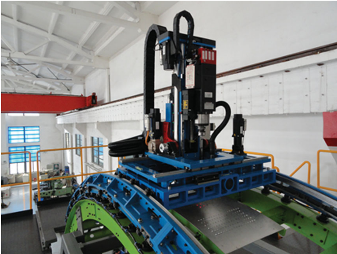
Fig. 1. The circumferential drilling machine developed at Zhejiang University.
