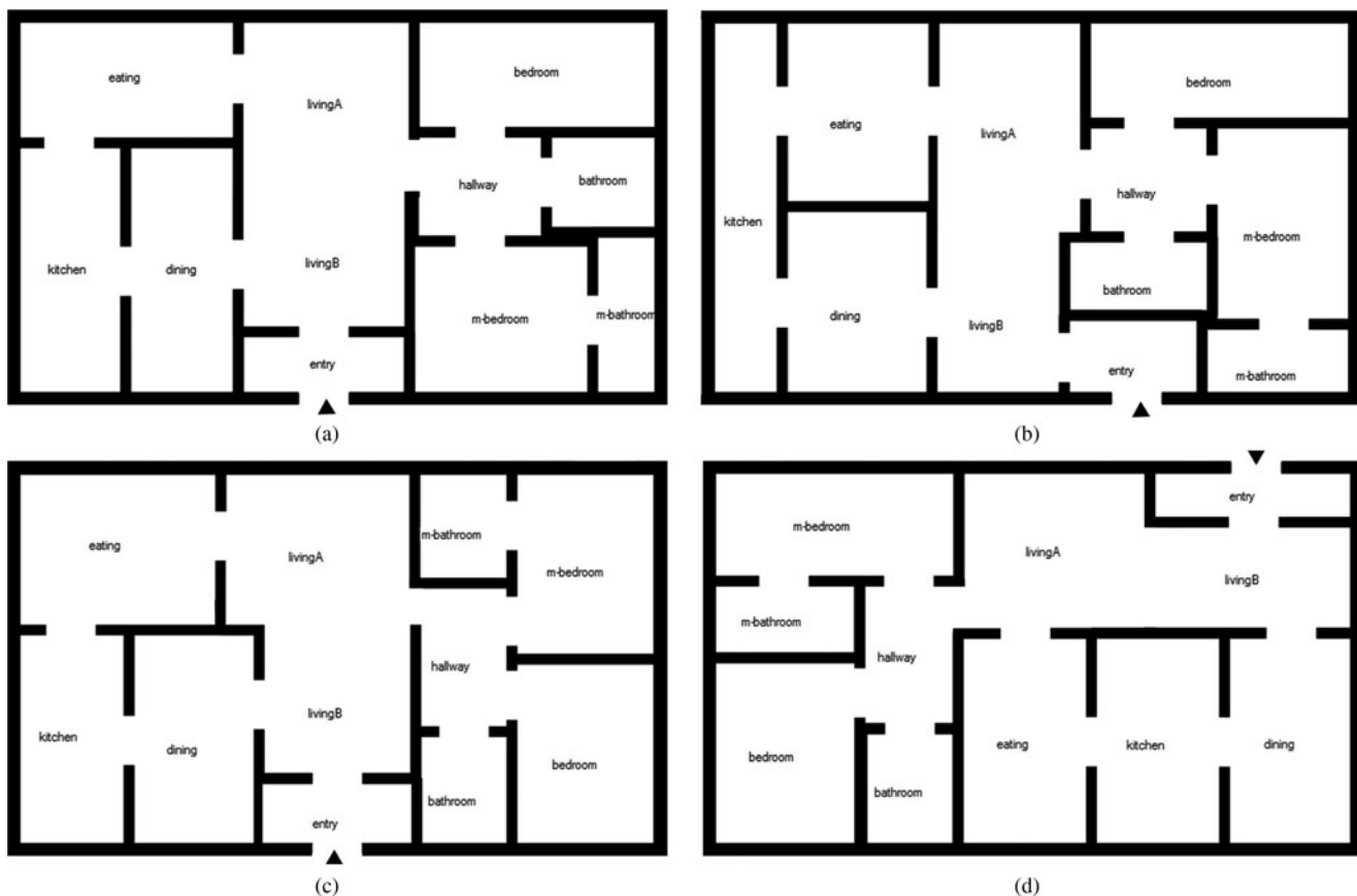
Fig. 10. Screenshot of four solutions for layout scenario 3 (11 rooms) found using the dense packing layout solver.
