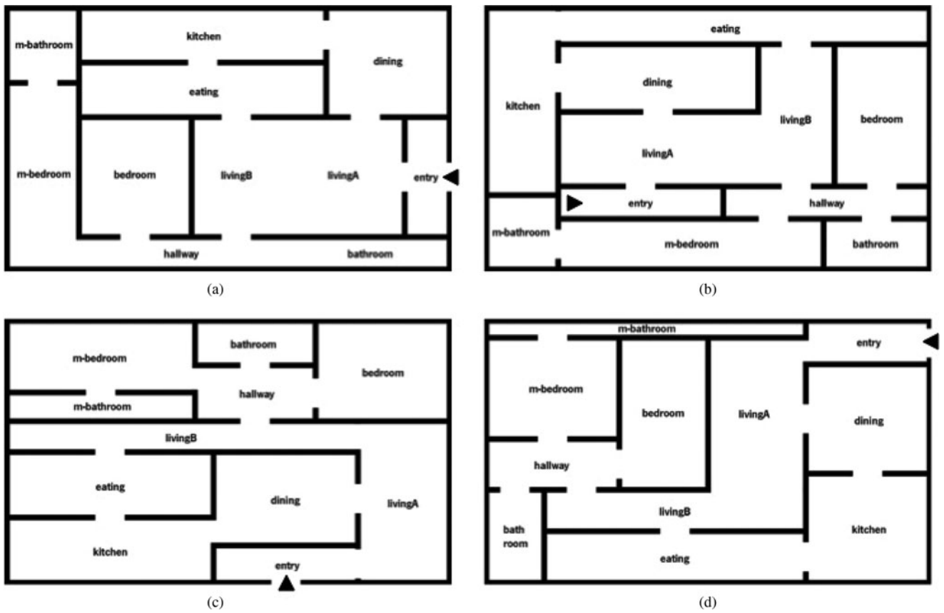
Fig. 11. Screenshot of four solutions for layout scenario 3 (11 rooms) generated by the subdivision layout solver.
