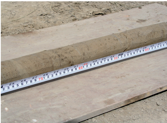
Fig. 2. a. The drilling site at PZS; b. The recovered aeolian loess core from the PZS site at depth of around 9 meter.
