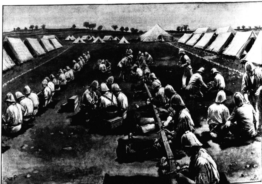
DRAWN BY WAL PAGET The men of the Royal Warwickshire Regiment are here shown altering the service bullet to the Dum-Dum pattern. This is done by filing a portion off the end. After a little practice the men become very proficient at the work. A number of "filers" are shown seated on the ground, with their legs under an inverted railway rail raised about eighteen inches from the ground on stones. Behind them are a certain proportion of "unpackers." The latter unpack the boxes of numbered ammunition, which are brought to them by carriers. FROM A SKETCH BY MAJOR G. W. COCKEY'S In front of the "filers" sit the "packers," who, as the altered ammunition is passed to them, after it has been gauged by an officer, replace the cartridges in their packages and refill the empty boxes. In this way eight boxes (4,500 rounds) can be altered and repacked in two hours and a half, if fifteen to twenty "filers" are employed, or roughly, about sixty cartridges a minute.
