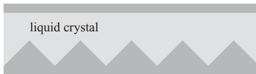
FIGURE 14. A typical periodic grating structure, which can support several stable director states.
