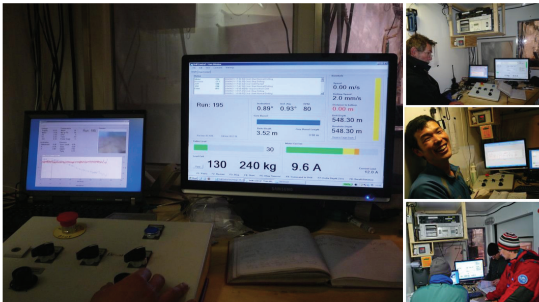
Fig. 9. The drill operator's winch console and control software made teaching new drillers easy and safe, with fine control and real-time monitoring and feedback from downhole parameters.
