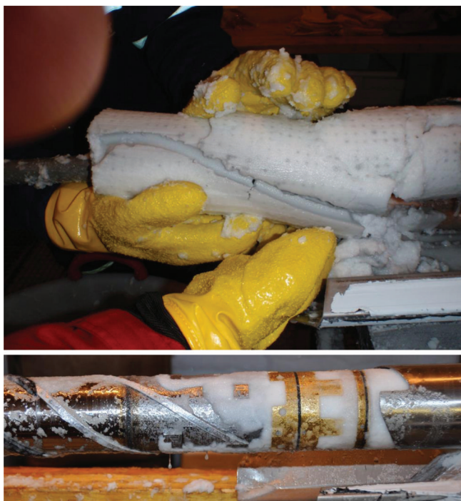
Fig. 12. Examples of chips packing in an unproductive way. Upper panel shows an example where drill fluid was forced to pass through the chips mass during a core break creating the channel. The dotted surface of the chips mass was formed by the small holes in the chip chamber body. Lower panel shows an example where the pump was completely packed and disengaged (May 2010).
