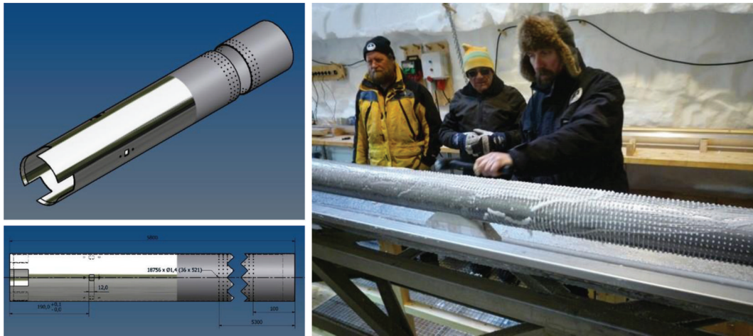
Fig. 5. The new 6 m long chip chamber designed for the NEEM drill. Includes fingers cut out of its tapered lower end which function to hold the piston pump stationary as the drill turns; 18 000 holes drilled along its body to increase the drill's filter capacity; and an adaptation for simple assembly with the outer core barrel which replaces the weld junction of previous versions (photograph June 2009).
