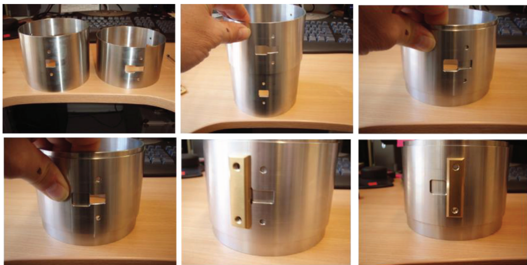
Fig. 6. Demonstration of the locking mechanism that couples the chip chamber to the outer core barrel. The tapered lower end of the chip chamber is fitted into the upper part of the outer core barrel and secured using a slotted locking mechanism with brass connectors. The brass connectors are then secured with a screw threaded into the core barrel wall.
