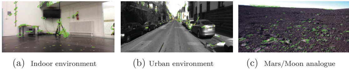
Fig. 3. SIFT image features with location covariances visualised via error ellipses.
