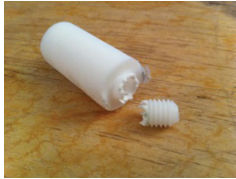
Fig. 11. PTFE liner failure. Source: http://forums.reprap.org/read.php?1,124652,124784 , photo by Pierre le Vrai.
