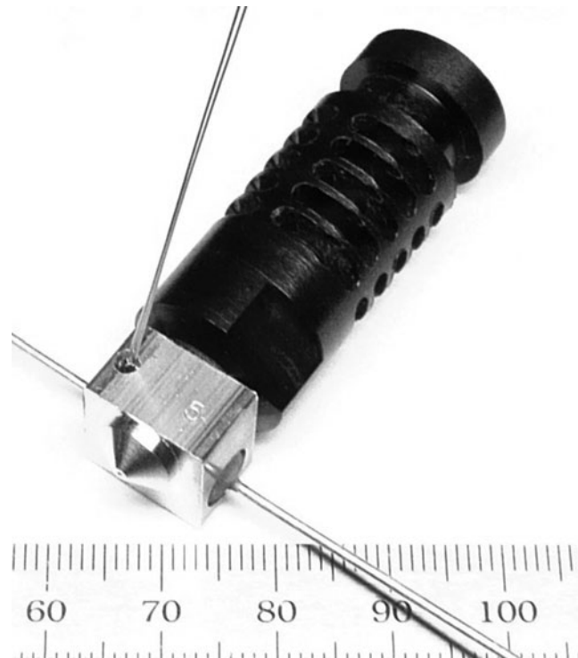
Fig. 8. J Head nozzle, PEEK filament guide (black), and aluminum heater block with resistors. Source: http://www.reprap.org/wiki/J_Head_Nozzle , author: Brian Reifsnyder.
