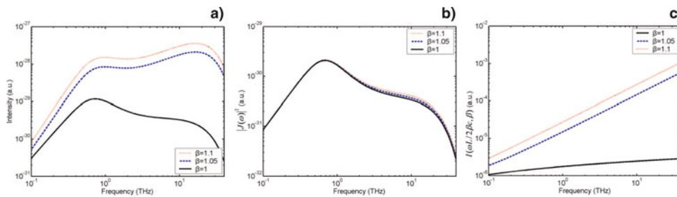
**Fig. 2.** (Color online) (a) The THz radiation spectrum, (b) the localized electron current term of dipole oscillation  $|J(\omega, \rho = 0)|^2$ , and (c) the conventional Cherenkov radiation term  $I(\omega L/2\beta c, \beta)$  versus the frequency when  $\beta = 1, 1.05$ , and  $1.1$ .
