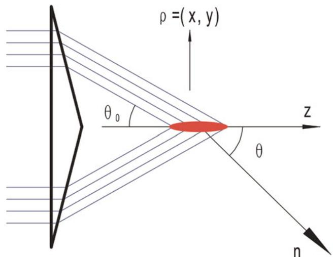
**Fig. 1.** (Color online) The scheme of THz wave generation by using axicon lens and the configuration of calculation.
