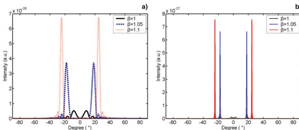
**Fig. 3.** (Color online) The angular distribution of the THz radiation at  $\omega = \omega_{pe}$  (a) and  $\omega = 10\omega_{pe}$  (b) when  $\beta = 1, 1.05$ , and  $1.1$ .
