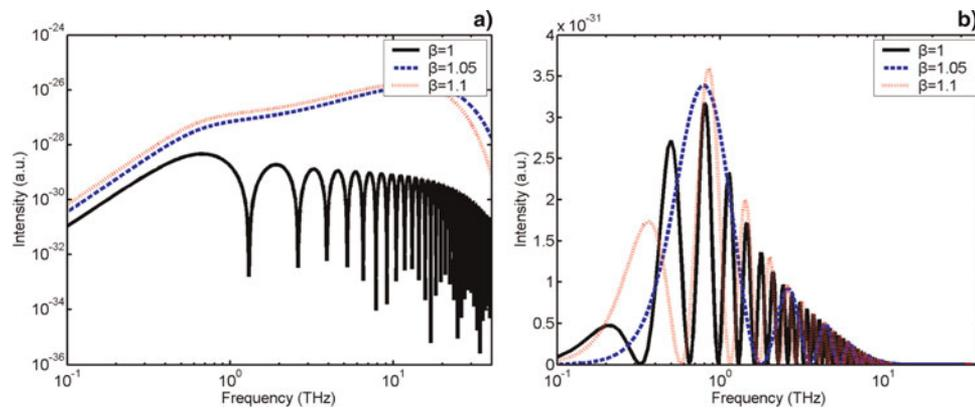
**Fig. 4.** (Color online) The spectrum at the angle of strongest radiation lobe (a) ( $\theta_{\max}$  for  $\omega = \omega_{pe}$ , as shown in Fig. 3a), and (b) at the angle vertical to the laser filament ( $\theta = 90^\circ$ ) when  $\beta = 1, 1.05$ , and  $1.1$ .
