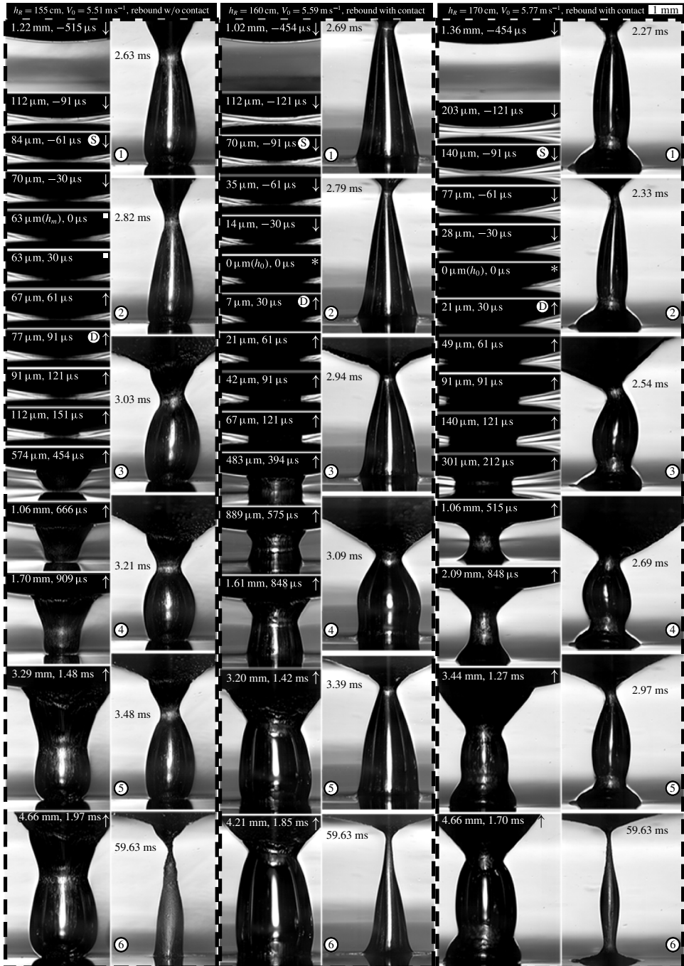
FIGURE 12. Side-view images of impacts onto a 5 mm thick layer of \nu_0 = 20\,000\,000 cSt silicone oil from h_r = 155 , 160 and 170 cm. R_0 = 10 mm, V_0 = 5.51 m s ^{-1} , 5.59 m s ^{-1} , 5.77 m s ^{-1} corresponding to St_0 = 9.31 \times 10^{-3} , 9.45 \times 10^{-3} , 9.75 \times 10^{-3} and De = 383 , 388, 401, respectively. The onset of shear-induced cavitation and cavitation by depressurization is marked by symbols (S) and (D), respectively. See also supplementary movie 2.
