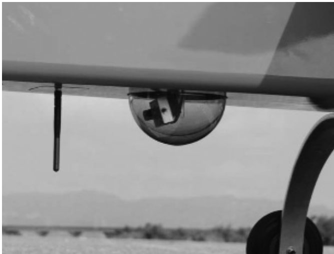
Figure 5. Onboard video camera and the wireless video transmission antenna.
