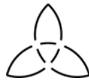
Fig. 11. Decomposition of the initial shape C of the trefoil grammar into six atoms.
