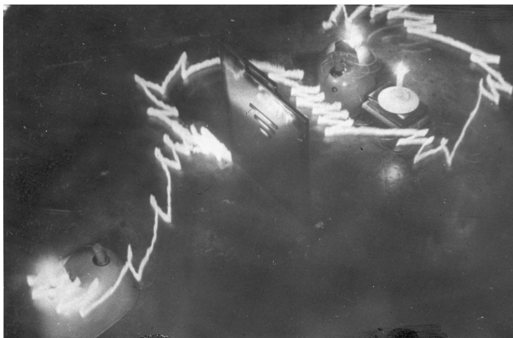
Fig. 5. Elsie demonstrates 'Pertinacity'. Initially distracted by the reflection of its own candle in the polished fire-screen, the robot eventually finds its way to the candle behind the screen.
