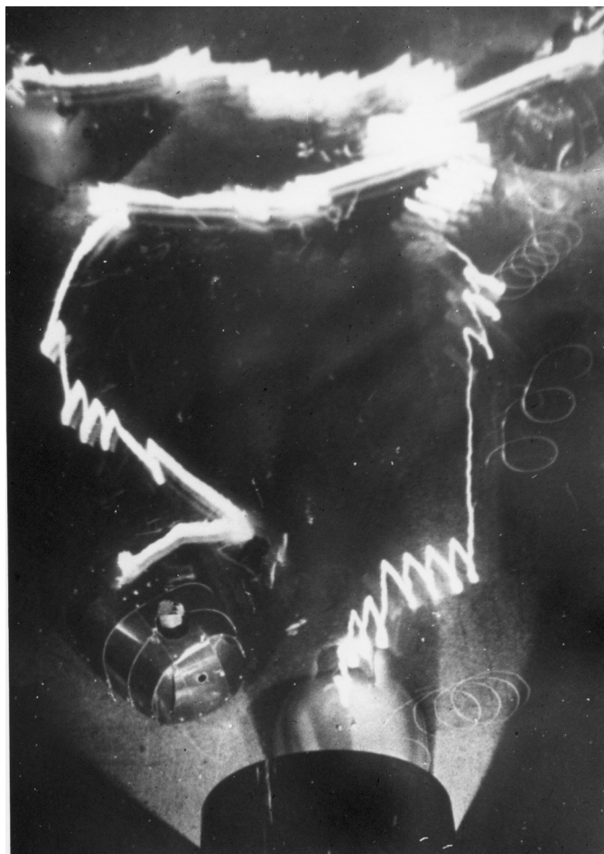
Fig. 4. A time lapse photograph of Elmer and Elsie, taken at Grey Walter’s house in 1949 or 1950, and showing the tortoises interacting with one another. The candles mounted on the backs of the robots trace out their trajectories; the fainter traces are made by the headlamps. Elmer, with the darker segmented shell, starts from the top right, and Elsie from the top left. The hutch is at the bottom of the picture.
