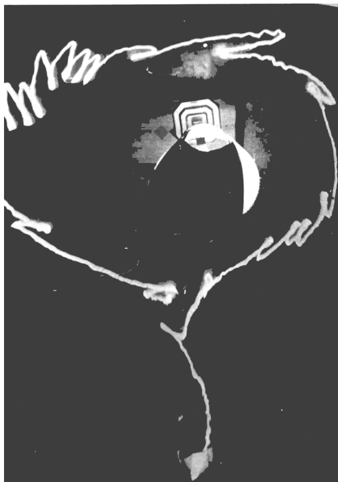
Fig. 8. Elsie demonstrates the 'Search for an Optimum' by approaching the lamp, and then circling round it at a distance.
