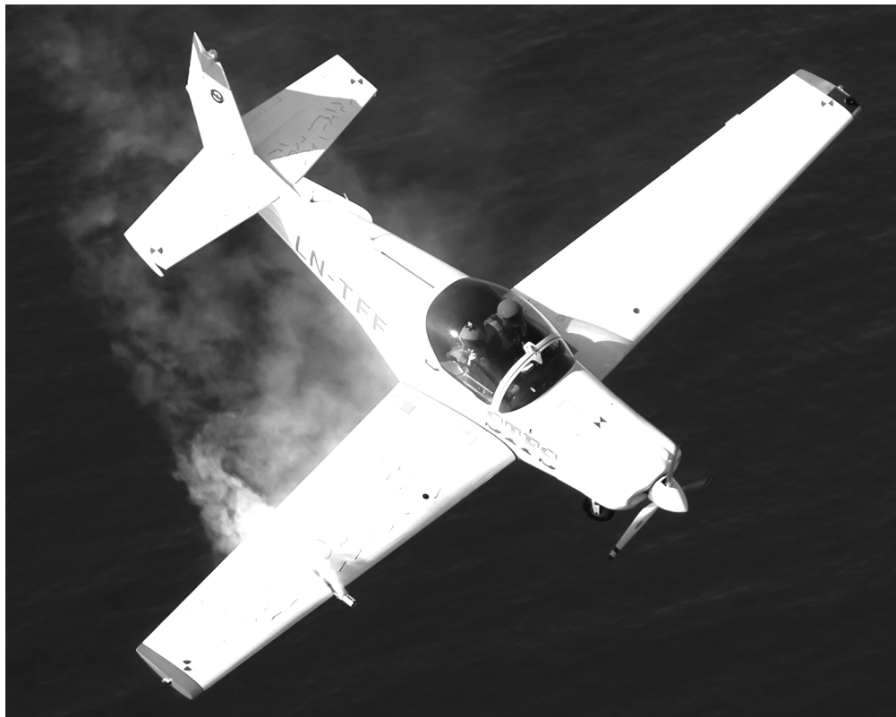
Figure 5. Smoke visualisation before the 1-turn point in the left spin.
