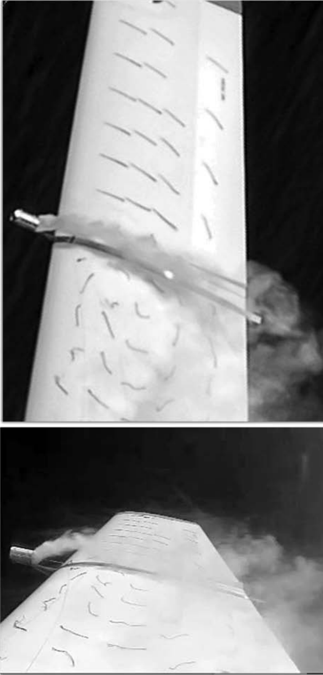
Figure 4. Smoke is pulled inwards by the USV as it moves towards the wing tip during the spin entry (from the \frac{1}{2} -turn point). The top and bottom images, from the helicopter chase and the cockpit camera respectively, are synchronised.
