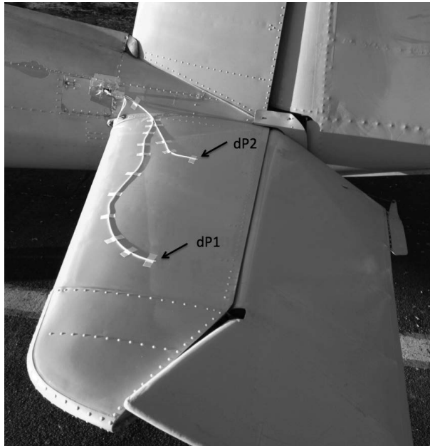
Figure 3. The modified Pitot-Static system circuit board was installed in the aft Saab Safir fuselage and the plastic tubes were routed on upper and lower surface to the desired points used for measurement (two points on the upper surface and two points on the lower surface). Tube marked dP1 was connected to the first, and dP2 was connected to the second differential pressure sensor.
