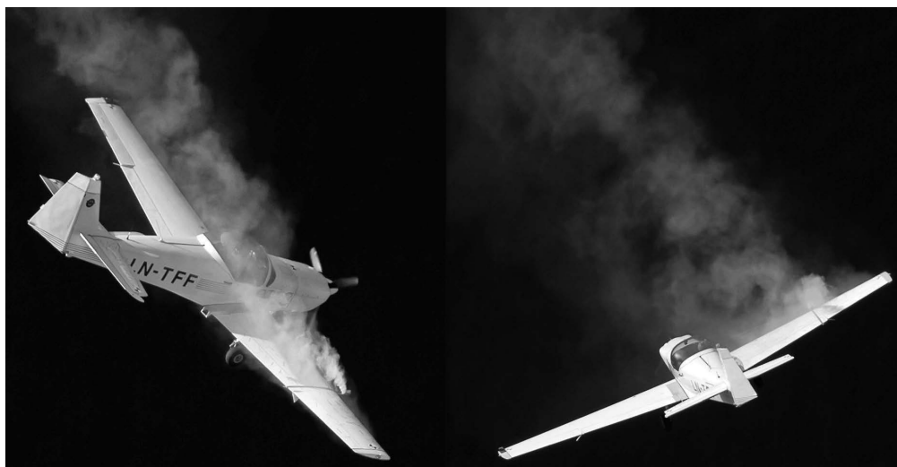
Figure 6. Before the 2-turn point (left image) in the spin, and after full right rudder was applied for the recovery at the 2-turn point (right image), smoke was visible towards the wing tip.
