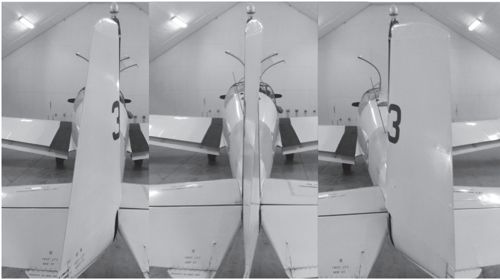
Figure 9. Pictures of the Saab Safir rudder showing full left, neutral and full right positions. Note the twisted rudder and the difference in rudder angle when displaced full left and full right.
