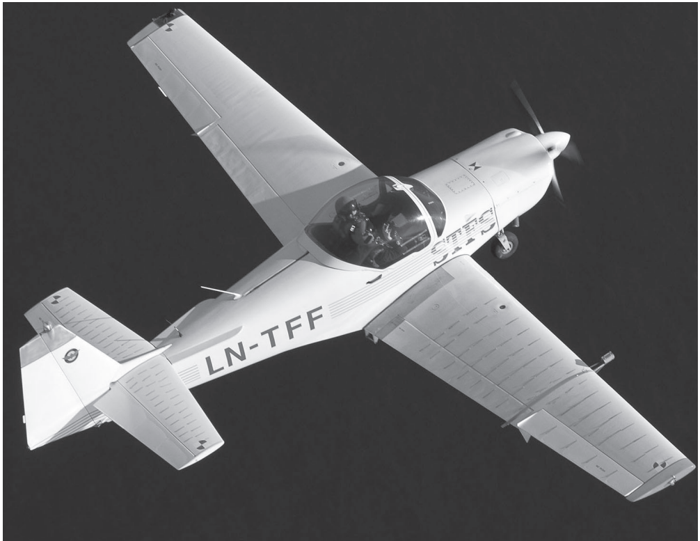
Figure 1. The Slingsby Firefly research aircraft in flight. Note the smoke boom attached to the wing, wool tufts on the right wing and also on the horizontal tail surfaces.
