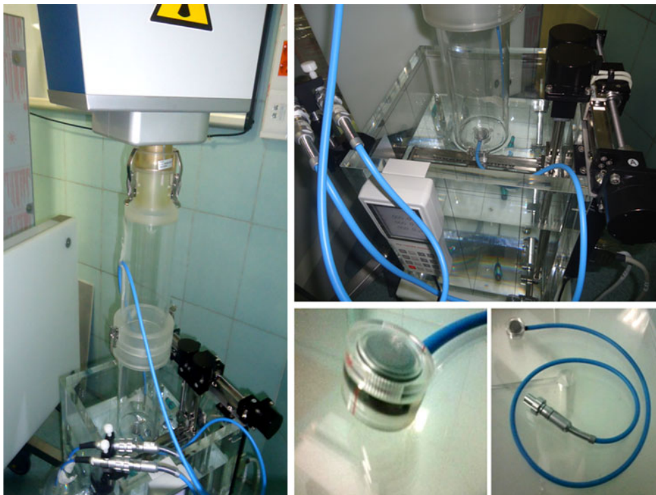
Figure 4. Experimental set-up view of absorbed dose measurement inside a MP3-XS water phantom using Advanced Markus ion chamber.
