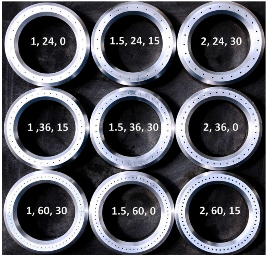
Fig. 3. Interchangeable drill heads; the numbers inside indicate diameter of the nozzles, the number of nozzles and angle from the vertical axis of the drill.
