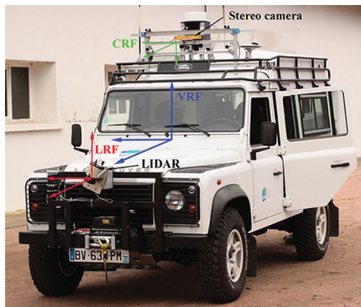
Fig. 2. The test platform employed in this research. It was made available by IRSTEA within the research activity connected with the Ambient Awareness for Autonomous Agricultural Vehicles (QUAD-AV) project, funded by the 2011 ICT-AGRI FP7 European Research Program.
