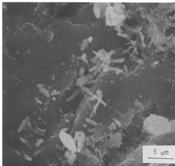
Figure 14. Scanning electron micrograph of large, secondary calcite with small, surface flakes of lithiophorite, goethite, and kaolinite.
