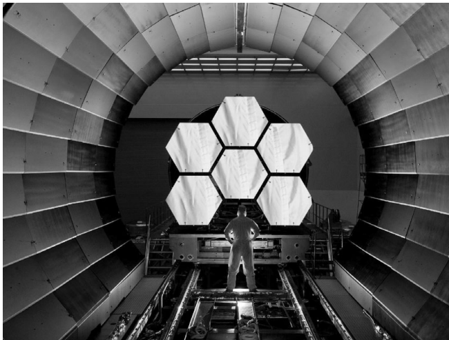
Figure 2. Six gold-coated JWST flight mirror segments prior to the start of cryogenic acceptance testing at the X-Ray Calibration Facility, located at the Marshall Space Flight Center.
