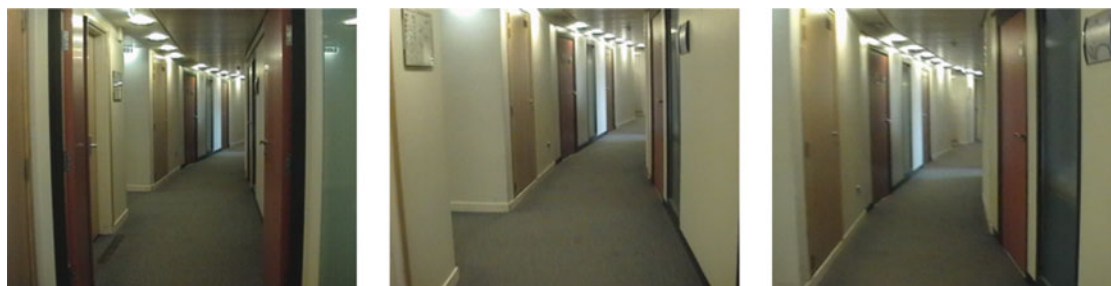
Fig. 16. Example of adding intermediate nodes in the Lip6Indoor dataset. Images 13 (Left) and 86 (Right) were added to the map at the first loop. Image 228 (Center) was added to the map the next time the camera visits the same place. As can be seen, image 228 is visually in-between the left and right images.
