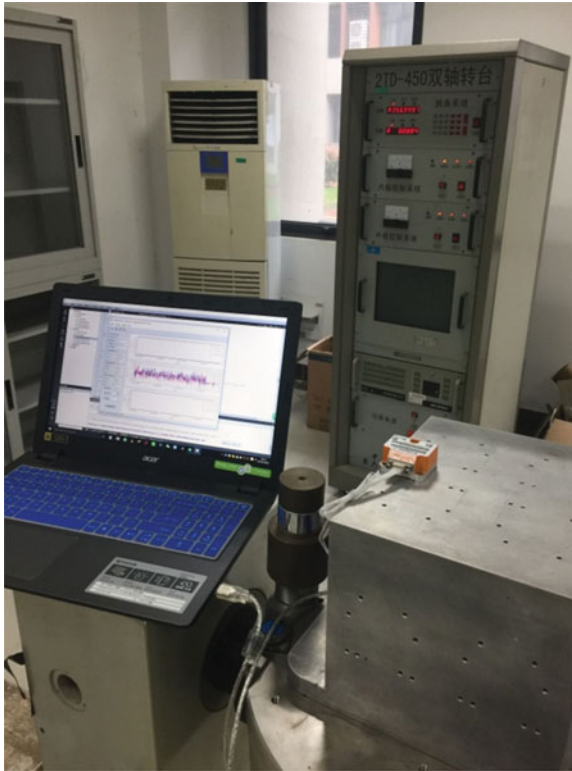
Figure 6. The MEMS IMU product STIM300 and its data acquisition equipment.
