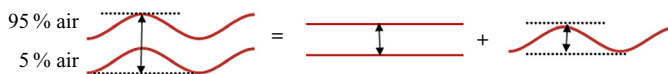
FIGURE 6. Schematics for the decomposition of the measured single-mode amplitude: half the width of the unperturbed interface and the amplitude of a sharp single-mode interface.
