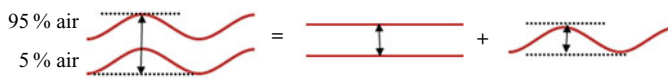
FIGURE 6. Schematics for the decomposition of the measured single-mode amplitude: half the width of the unperturbed interface and the amplitude of a sharp single-mode interface.
