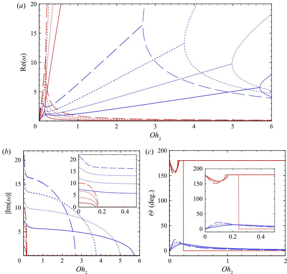
Figure 7. Dependence of (a) the damping rate  $\text{Re}(\omega)$ , (b) the angular frequency  $|\text{Im}(\omega)|$  and (c) the phase difference  $\Theta$  on the Ohnesorge number of the shell  $Oh_2$ , for the case of a viscous liquid shell,  $l = 2$  (solid), 3 (dotted), 4 (short dashed) and 5 (long dashed),  $a = 0.8$ . Blue curves, the in-phase mode; red curves, the out-of-phase mode. The insets in panels (b) and (c) show the details at small values of  $Oh_2$ .
