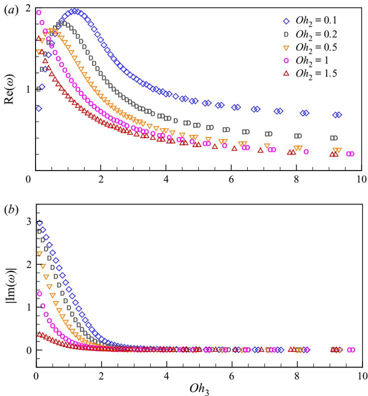
Figure 15. Variation of (a) the damping rate  $\text{Re}(\omega)$  and (b) the angular frequency  $|\text{Im}(\omega)|$  of the in-phase mode with the Ohnesorge number of the host fluid  $Oh_3$  for various values of the Ohnesorge number of the shell fluid  $Oh_2$ . The case of a viscous compound droplet immersed in a viscous host fluid,  $l = 2$ ,  $a = 0.8$ ,  $\rho_{r1} = 1$ ,  $\mu_{r1} = 1$ ,  $\gamma_r = 1$ ,  $\rho_{r3} = 1$ .
