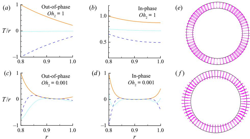
Figure 6. (a–d) Distribution of the normalized eigenfunction of the vorticity,  $T/r$ , along  $r$ , for the case of a viscous liquid shell,  $l = 2$ ,  $a = 0.8$ . The solid, dashed and dotted lines denote the absolute value, the real part and the imaginary part of the eigenfunction, respectively. The velocity fields of (e) the out-of-phase mode and (f) the in-phase mode at the initial time  $t = 0$ .
