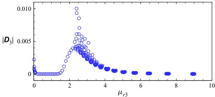
Figure 18. The absolute value of  $D_3$ , i.e.  $|D_3|$ , obtained by substituting the eigenvalues in figure 14(c) into the determinant  $D_3$  in (C1), versus the host to shell viscosity ratio  $\mu_{r3}$ .
