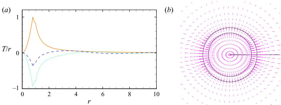
Figure 16. (a) The eigenfunction of the vorticity,  $T/r$ , along  $r$  (solid, the absolute value; dashed, the real part; dotted, the imaginary part) and (b) the velocity field of the in-phase mode at the initial time  $t = 0$ , for the case of a viscous compound droplet immersed in a viscous host fluid,  $l = 2$ ,  $Oh_2 = 1$ ,  $a = 0.8$ ,  $\rho_{r1} = 1$ ,  $\mu_{r1} = 1$ ,  $\gamma_r = 1$ ,  $\rho_{r3} = 1$ ,  $\mu_{r3} = 1$ .
