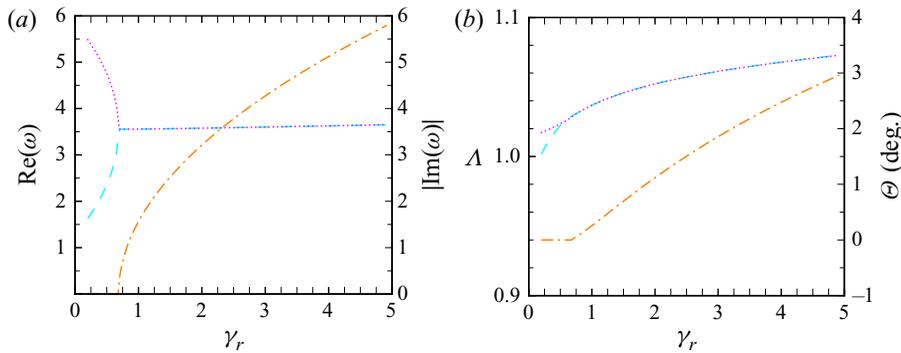
Figure 11. Influence of the interfacial tension coefficient ratio  $\gamma_r$  on (a) the damping rate  $\text{Re}(\omega)$  (dotted and dashed) and the angular frequency  $|\text{Im}(\omega)|$  (dash-dotted) and (b) the amplitude ratio  $\Lambda$  (dotted and dashed) and the phase difference  $\Theta$  (dash-dotted) of the in-phase mode of a viscous compound droplet in a vacuum,  $l = 2$ ,  $Oh_2 = 1$ ,  $a = 0.8$ ,  $\rho_{r1} = 1$ ,  $\mu_{r1} = 1$ .
