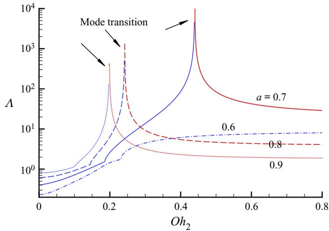
Figure 4. Variation of the amplitude ratio  $\Lambda$  with the Ohnesorge number of the shell  $Oh_2$  for different values of the radius ratio  $a$ . The case of a viscous liquid shell,  $l = 2$ . Only the result of the upper aperiodic branch of the out-of-phase mode is plotted. The arrows indicate the locations where the transition of mode from out of phase (blue curves) to in phase (red curves) takes place.
