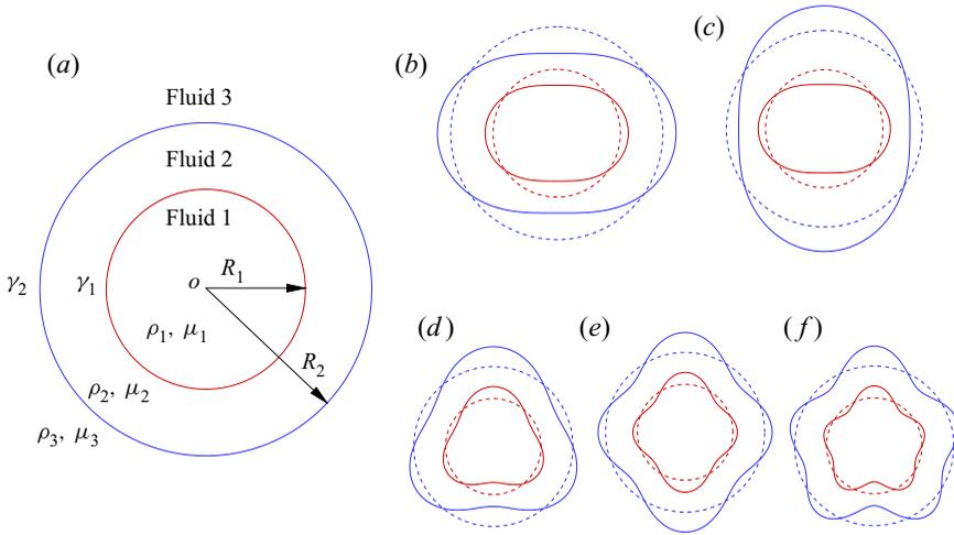
Figure 1. (a) Schematic of the theoretical model. (b) The in-phase deformation and (c) the out-of-phase deformation of the interfaces, for the fundamental mode  $l = 2$ . (d–f) The in-phase deformations for the higher-order modes  $l = 3, 4$  and  $5$ , respectively.
