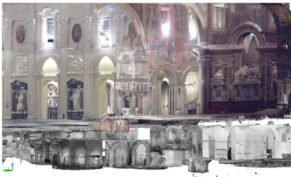
Fig. 1. A cutaway image of the Archbasilica of St John Lateran derived from laser scans by the Lateran Project. This derives from the integrated 3D model of the Lateran used by Project members to facilitate analysis of the key spatial relationships within the complex.
