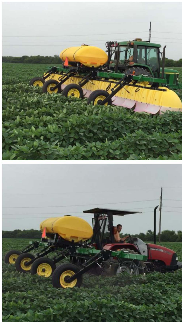
Figure 1. Broadcast Redball hooded sprayer with a continuous shield (top) and broadcast Redball open sprayer (bottom) (Wilmar Manufacturing LLC, Benson, MN).
