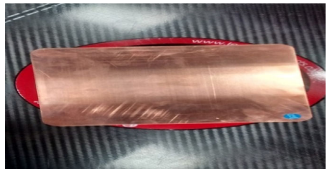
Figure 8. TOR 18FG phantom with 1-mm Cu plate position.
