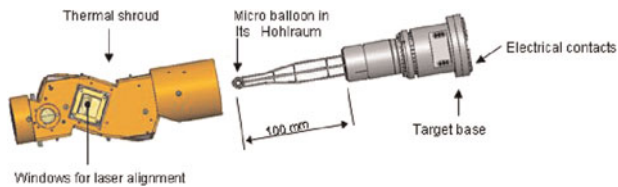
Fig. 1. (Color online) A view of the cryogenic target with its thermal shroud.
