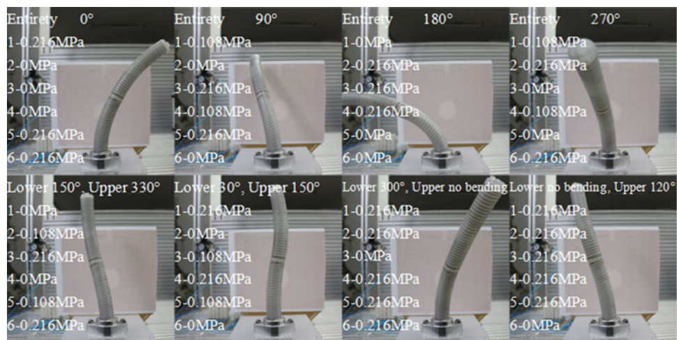
Fig. 19. Dual-segment soft robot experiments (“entirely,” “upper,” and “lower” indicate respectively the bending direction of the whole soft robot, the upper segment, and the lower segment, 1–3 indicate the lower motion-driving chambers, 4–6 indicate the upper motion-driving chambers, and the value after the number indicates the air pressure).
