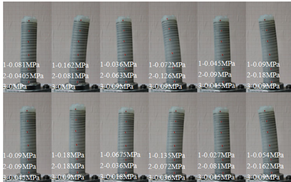
Fig. 18. Multi-chamber driving bending experiment.
