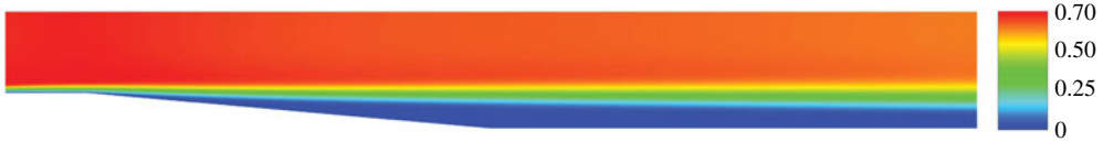
FIGURE 2. (Colour online) Mach number contours at steady state.
