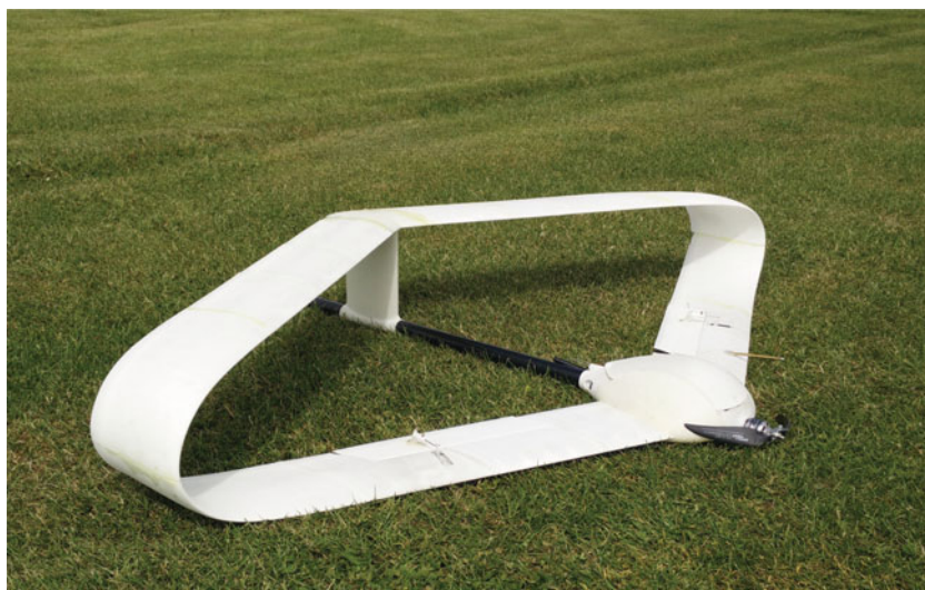
Figure 19. The SLS fabricated version of Aircraft 1.
