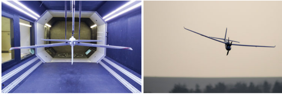
(a) Wind-tunnel testing the reference aircraft.
