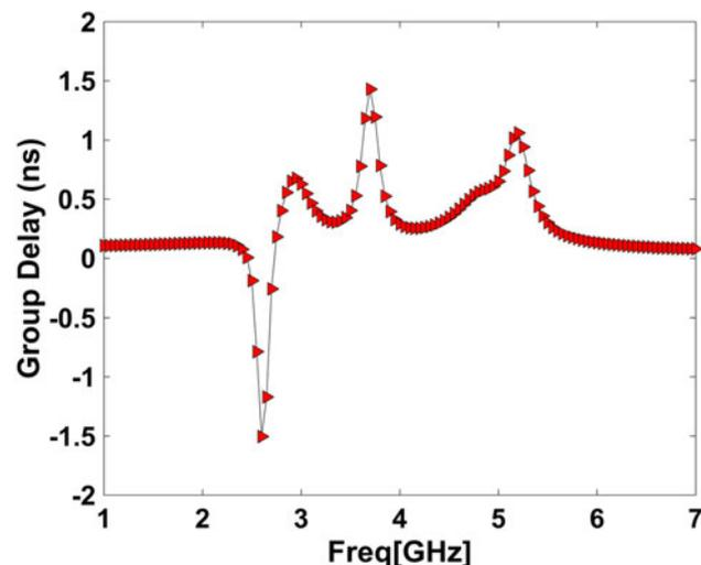
Fig. 3. Simulated group delay for the proposed single antenna.
