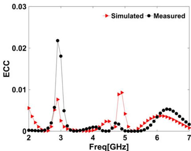
Fig. 10. Simulated and measured ECC curve for the proposed MIMO antenna.
