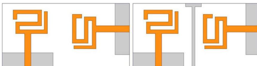
Fig. 8. MIMO antenna with and without T-bar parasitic element.
