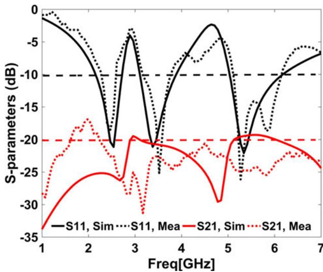
Fig. 13. Simulated and measured  $S_{11}$  and  $S_{21}$  for the proposed MIMO antenna.
