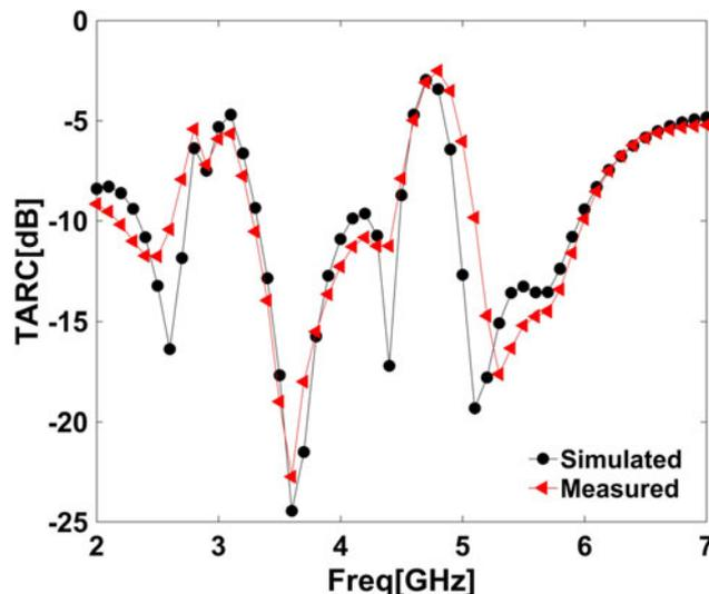
Fig. 11. Simulated and measured TARC curve for the proposed MIMO antenna.
