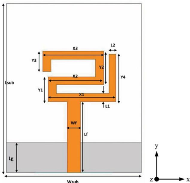
Fig. 1. The proposed single antenna configuration and parameters.
