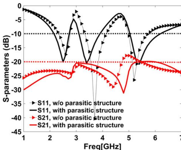
Fig. 9. MIMO antennas  $S_{11}$  and  $S_{21}$  with and without T-bar parasitic element.
