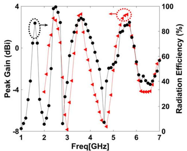
Fig. 14. Simulated peak gain and radiation efficiency for the proposed MIMO antenna.
