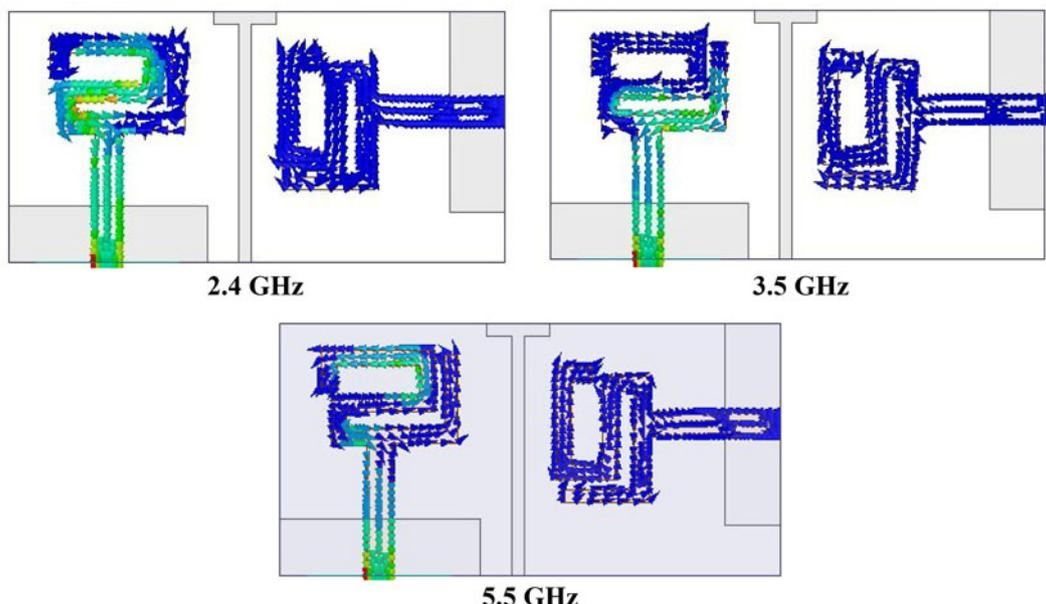
Fig. 7. Surface current distribution on the proposed MIMO antenna.
