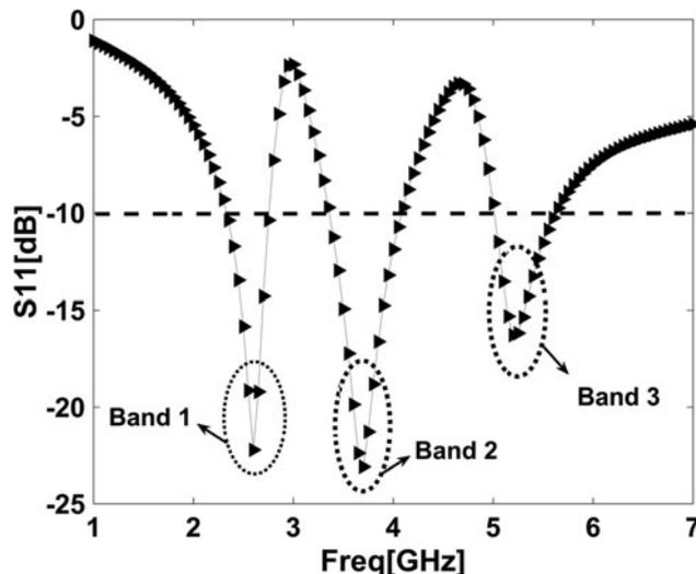
Fig. 2. Simulated S<sub>11</sub> curve for the proposed single antenna.
