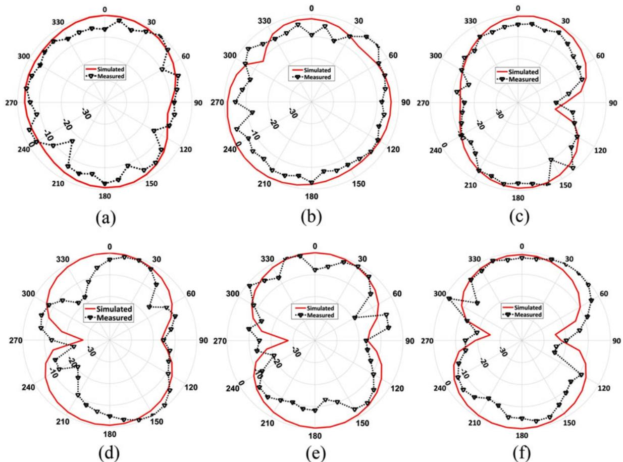
**Fig. 16.** The radiation pattern of the proposed MIMO antenna in (a) 2.4 GHz, (b) 3.5 GHz, (c) 5.5 GHz in the Y-Z plane and (d) 2.4 GHz, (e) 3.5 GHz, and (f) 5.5 GHz in the X-Z plane.
