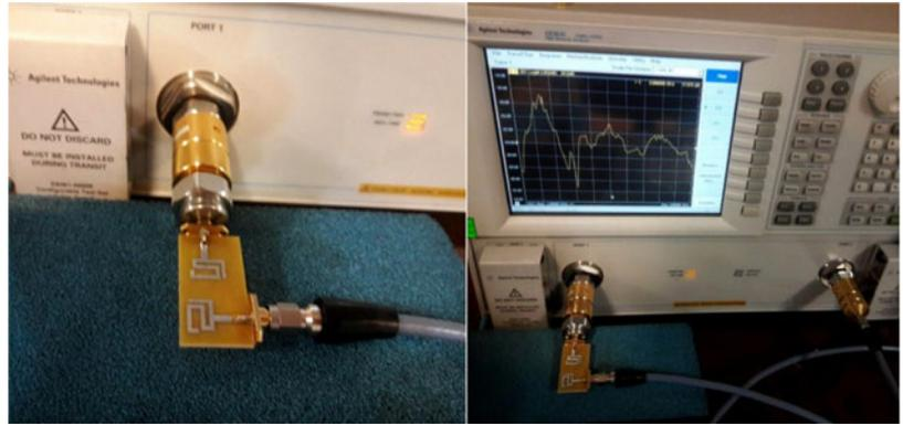
Fig. 12. Fabricated MIMO antenna under measurement process.
