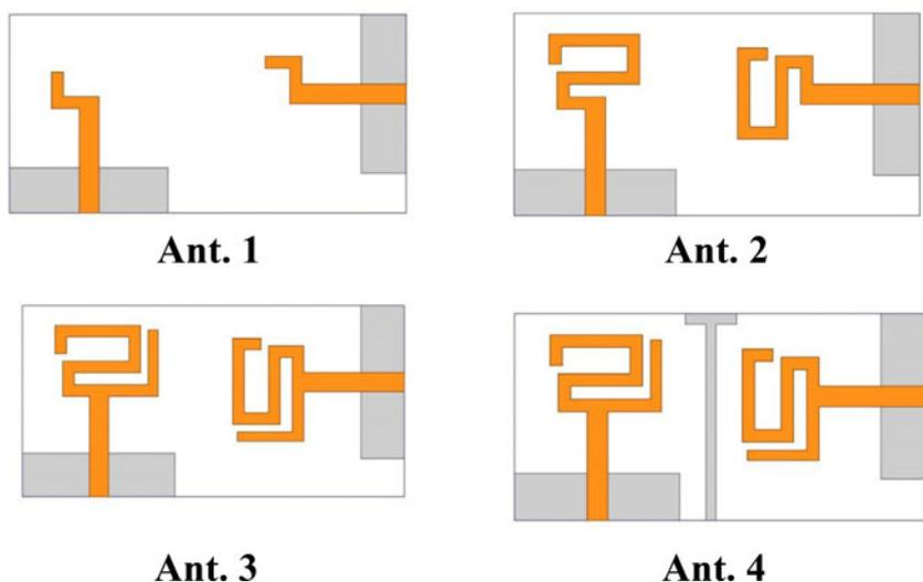
Fig. 5. The MIMO antenna design process.
