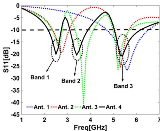
Fig. 6.  $S_{11}$  curves for different antennas in the MIMO design process in Fig. 5.
