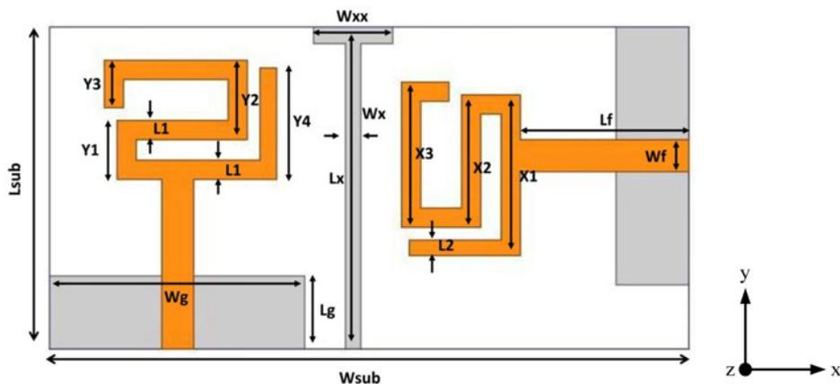
Fig. 4. Configuration of the proposed two-element MIMO antenna.
