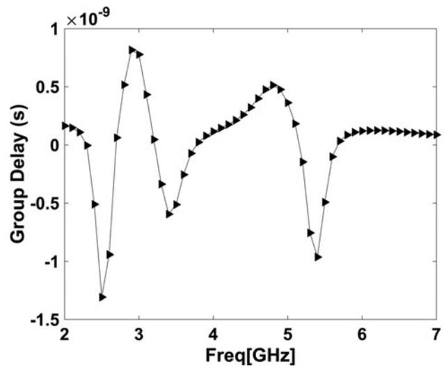
Fig. 15. Simulated group delay for the proposed MIMO antenna.
