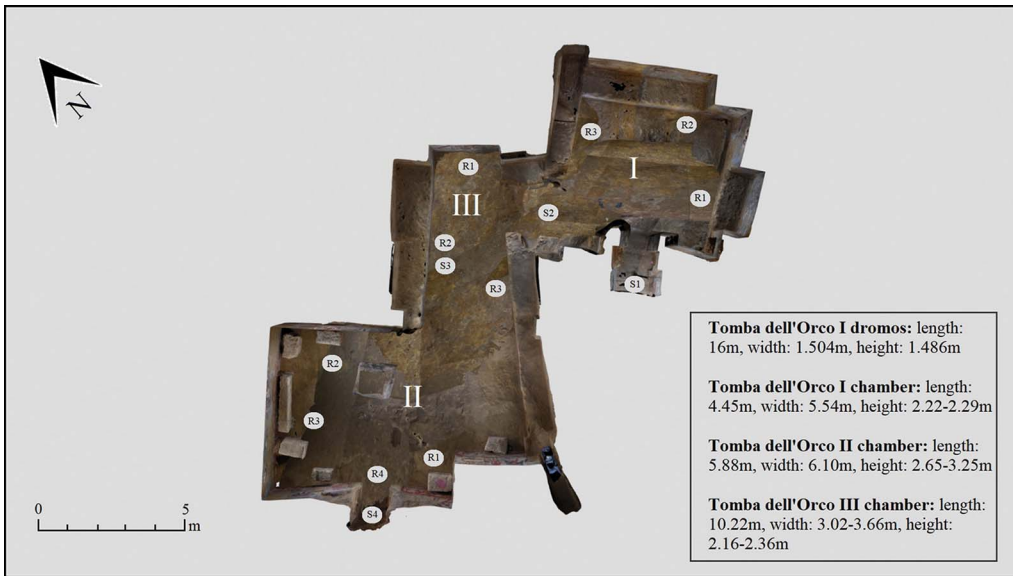
Figure 6. Acoustic site plan of the Tomba dell'Orco I, II and III: S1–4 represent sound sources; R1–4 represent sound receiver points (model by J.K. Ortoleva).
