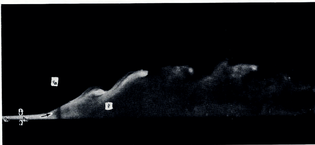
Fig. 8. View of a moving observer of a vertical slice of the head of a gravity current (or of a thermal) developing in the presence of a thin layer on the floor of density \rho_N = \rho_0 ( \Delta\rho_0/\rho_0 = 1\% ). It is seen that most of this thin dense layer is lifted up above the head. \alpha = 10^\circ .
