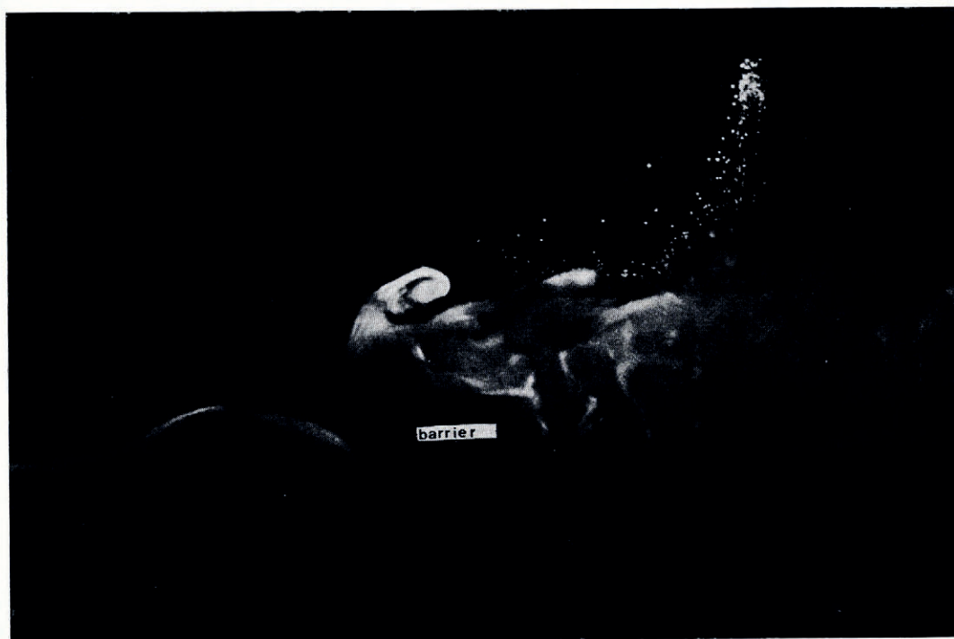
Fig. 9. View by a moving observer of a vertical slice of a gravity current when it traverses an obstacle of a wedge angle of 30^\circ . The hydrogen bubble trains indicate an acceleration above the obstacle. Here, a dense layer was present on the floor, but the phenomena are the same without such a layer ( \Delta\rho_0/\rho_0 = 1\% , \alpha = 10^\circ ).
