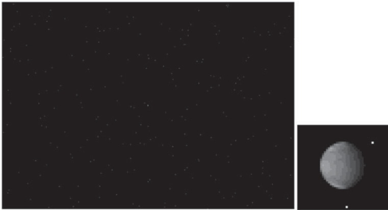
Figure 11. Simulated image for the spacecraft-to-Mars distance 10^7 \text{ km} . (left) total image on the image plane, (right) locally magnified Mars image.
