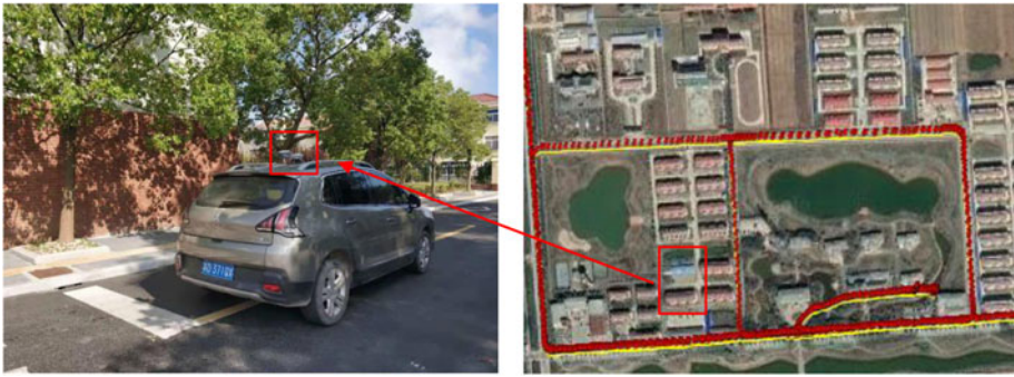
Figure 8. The vehicle used to perform the mission (left) and the main trajectory of the test (right). The red rectangle in the right picture represents the position of the GNSS receiver (left).
